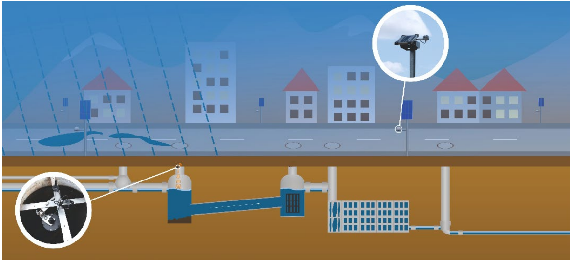
Figure 1. Schematic diagram of the monitoring of decentral stormwater treatment system
